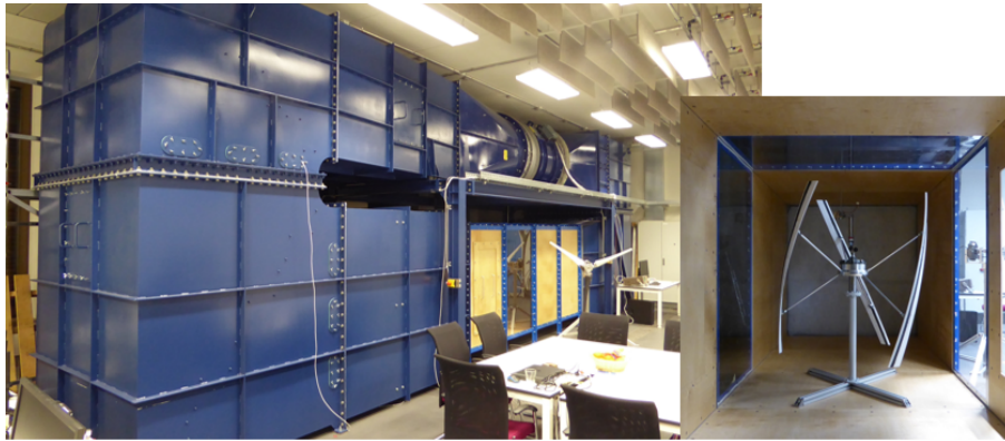
Figure 5 Low speed wind tunnel with test-rig and installed VAWT prototype
